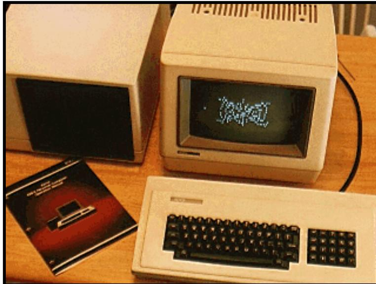
The Xerox 820-II is a powerful 64k CP/M machine. The entire computer is in the monitor except the I/O devices --disk drives, keyboard, etc. Upon first powering up the 820, you have a choice of loading CP/M, booting a dumb terminal, or booting a text editor.
