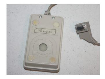
The original Amiga 1000 mouse had a large angled connector designed to fit snugly into the side connector of the Amiga case. When you see one of these connectors, you can be sure you are looking at an Amiga mouse.
