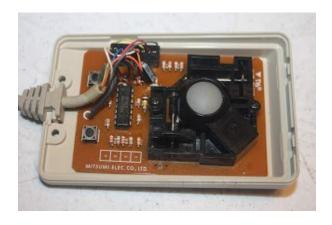
The later boards on the 1351 and Amiga mouse respectively, pictured above, have their components consolidated to a single board. The later 1351s don't seem to have any resisters along the left-hand-side of the board, while the later Amiga mice always do -- either three or five, depending on revision.
