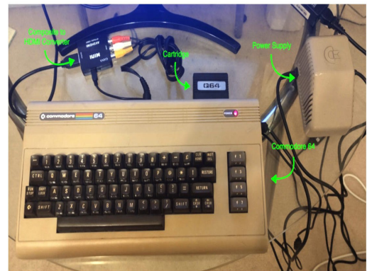
Figure 2: The experimental setup – a Commodore 64 is connected to a monitor through a composite video to HDMI converter, with the code cartridge inserted into the expansion port.
