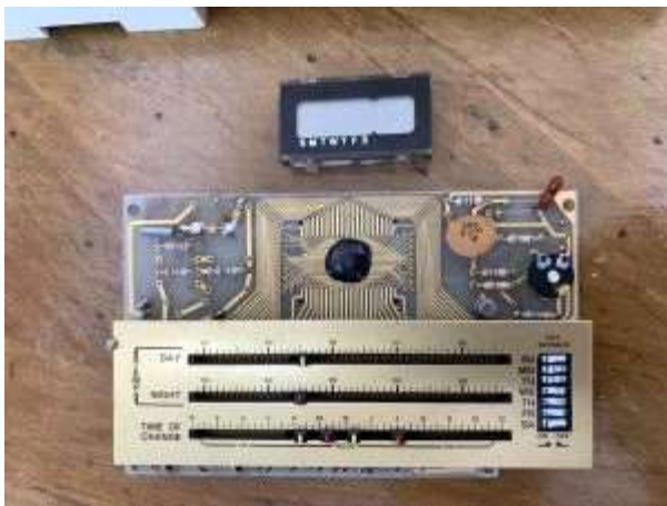
LSI chip secured to the board with blob of epoxy.
